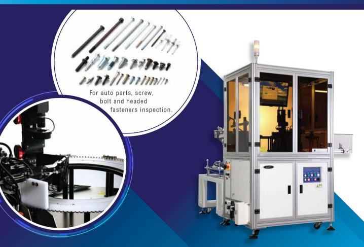
Continues rotating platform design, high speed inspection Innovative 360° thread damaged inspection design
